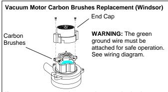
If armature commutator is grooved, extremely pitted or not concentric, the motor will need to be replaced or sent to a qualified service center.
